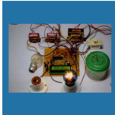
Transformer Protection System Project
